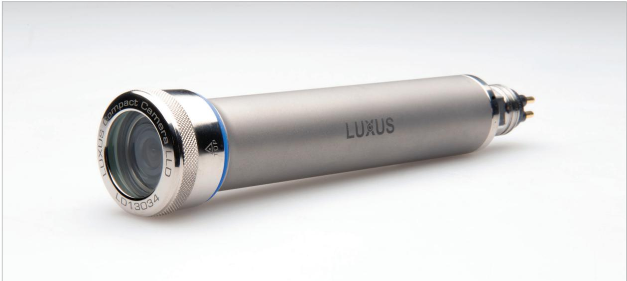
The LUXUS compact long line driver camera is a LUXUS compact camera fitted with a video signal amplifying unit. This unit increases the signal and compensates losses when the camera is used with extensive cable lengths for applications that do not involve telemetry.
